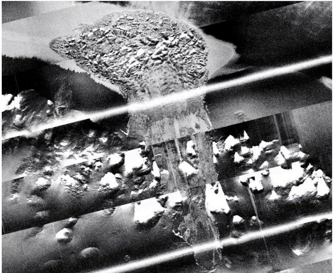
probably an undersea landslide is shown here. Several sonar passes were made over this area with each swath overlapping. After the REMUS collected the data, Jeff merged it together with navigation to make a mosaic, yielding the composite image shown here.
